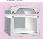
26-gauge stainless steel finishing liner, bonded to interior of both base and cover, and matching stain-less steel cover shield pro-vide a brilliant, durable and corrosion resistant finish.
